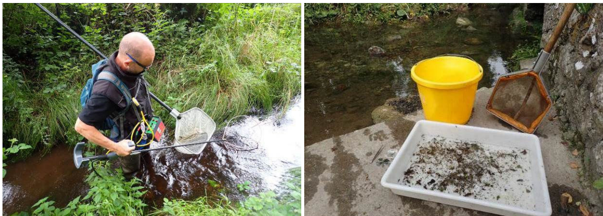
Plate 1: Electrical fishing sampling apparatus employed during the on-site investigations (left). Macroinvertebrate sampling kit used during biological water quality assessment (right).
